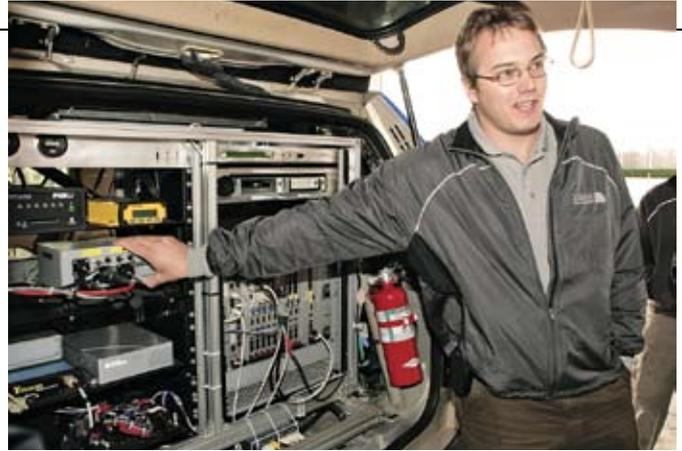
Chris Urmson, Director of Technology for Tartan Racing, shows the computers and electronics that are embedded in the Tartan Racing vehicle. The rear cargo area also includes a safety system that allows the vehicle to be stopped via a radio signal, if needed.
