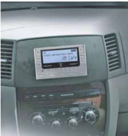
VoiceBox and XM Radio are using DSP to integrate voice control and data stream decoding.
