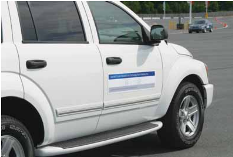
Vehicles equipped with DSRC, first demonstrated by DaimlerChrysler, can communicate directly with one another and the infrastructure around them using wireless local area network technology.
