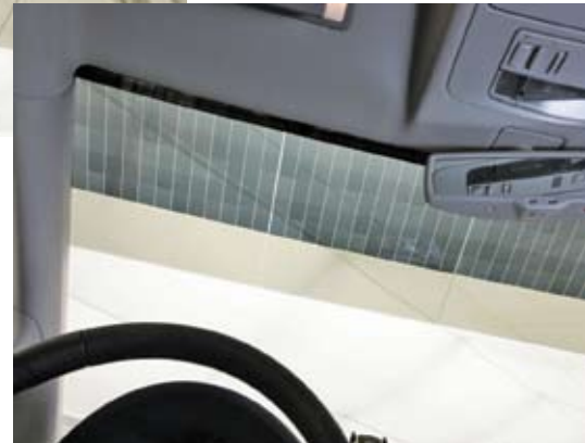
In normal operation, the electronic sun visor blackens only a spot on the windshield that's necessary to keep sunlight from blinding the driver. However, it can also blacken a large upper area of the windshield.
