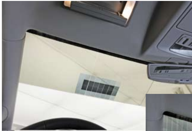
In normal operation, the electronic sun visor blackens only a spot on the windshield that's necessary to keep sunlight from blinding the driver. However, it can also blacken a large upper area of the windshield.
