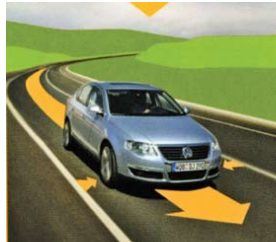
VW's Integrated Lateral Guidance system uses camera analysis of road and lane markings and a computer to control steering in the event an inattentive driver does not make the necessary adjustments to keep the car in lane.
