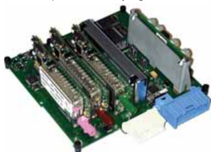
Hirschmann has developed a hybrid receiver for mobile TV reception in motor vehicles.
