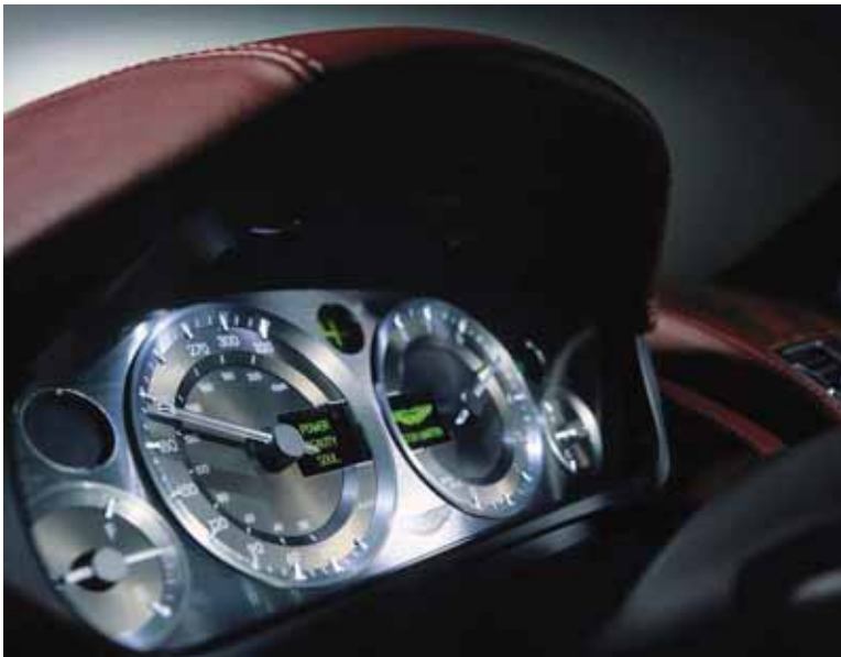
The instrumentation cluster of the new Aston Martin DB9 features the first automotive application of OLED technology.
