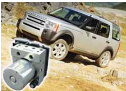
The Land Rover Discovery's Bosch-supplied ESP improves stability both on- and off-road.
