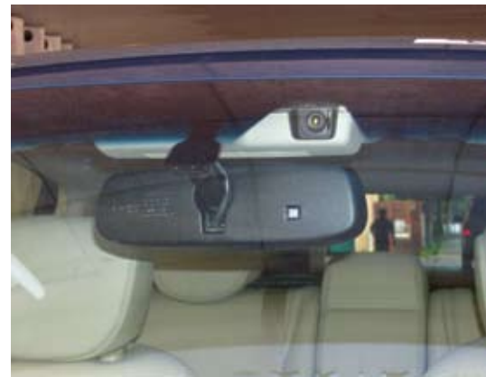
Infiniti's lane-departure-prevention system uses a forward-view camera above the rearview mirror to analyze roads for lane markings, whether they are in-use markings or those from discontinued lanes.
