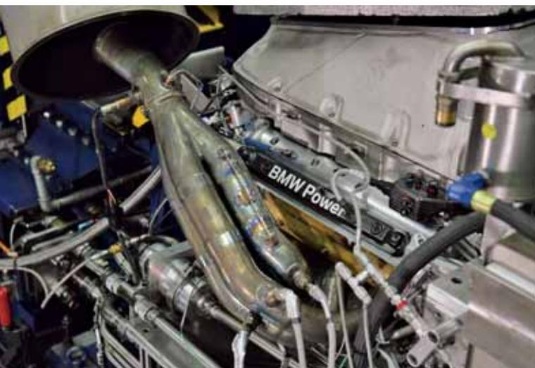
Vibrations from the V8s, which worsen in the heart of the power band, require not only reinforced engine parts, but also strengthened accessory mounts, brackets, and other attachments on the car so they can withstand the punishment over the course of a race. Shown is the new BMW P86 F1 engine during dyno testing.
