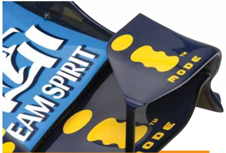
To make F1 cars less sensitive to the disruption of airflow by the car ahead, rules makers have raised the front wings to lessen their effectiveness. Teams such as Renault have responded with biplane wing elements designed to recover some of the downforce lost when the main element was raised away from the road.
