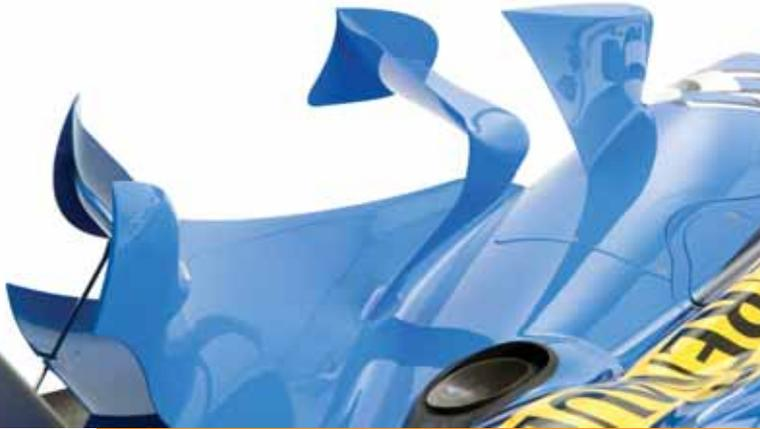
Increasingly, minimizing drag and maximizing downforce means managing airflow not just around the body, but away from the tires and toward the wings, as illustrated by these appendages on the Renault R26.
