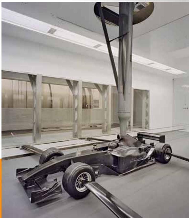
Extensive wind tunnel testing of 60% scale models helped teams such as BMW Sauber F1 minimize drag by testing the benefits of the smaller radiators permitted by the V8 engine's reduced cooling requirements.
