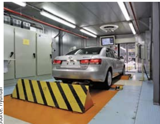
A dynamometer check is one of the final steps in vehicle production.
