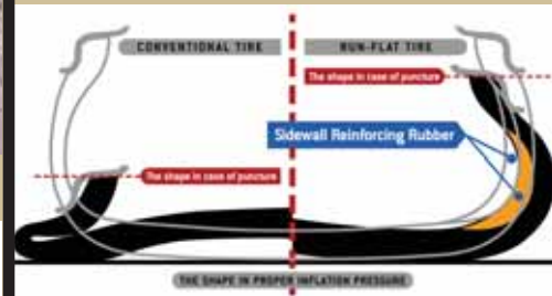
Bridgestone's run-flat tire technology has reinforced sidewalls
