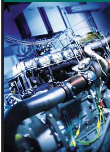
Heavy-duty diesel undergoing dyno testing
