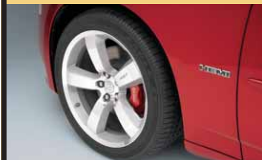
Dodge Charger SRT8 20-in forged aluminum wheels and high-performance Goodyear tires
