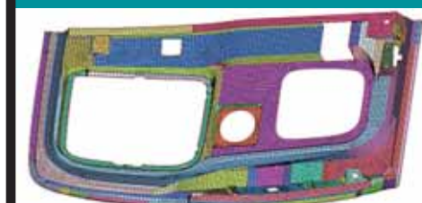
Detailed model of door inner panel
