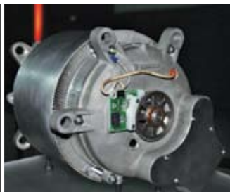
Tesla builds its own 185-kW electric motors using copper windings for maximum power density.
