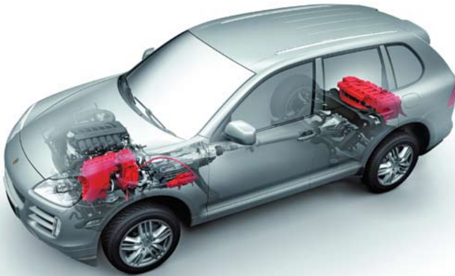
Porsche's parallel full hybrid Cayenne can be powered only by the electric motor at speeds up to 120 km/h (75 mph).
