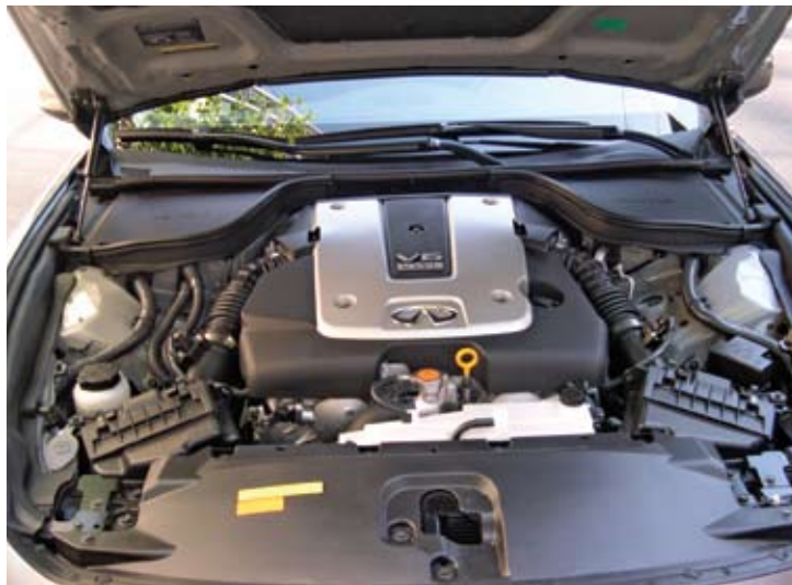
The G37's refreshed V6 moves up to 3.7 L with a small change in stroke, and dual throttle bodies fed by separate air cleaners are used to enhance performance.
