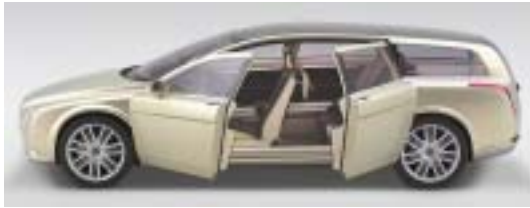
Volvo's Versatility Concept Car has no B-pillar and an aft-hinged rear door that reveals a simple but high-tech interior.
