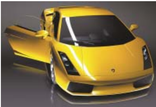
The Lamborghini Gallardo uses aluminum spaceframe construction.
