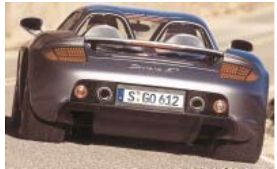
Porsche's Carrera GT has a 450-kW (603-hp) V10 and twin detachable carbon fiber roof shells.
