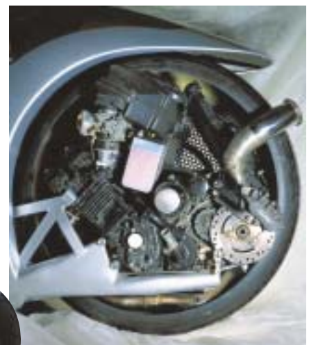
Sbarro showed a motorcycle concept with an engine inside its rear wheel and a sci-fi three-wheel concept.
