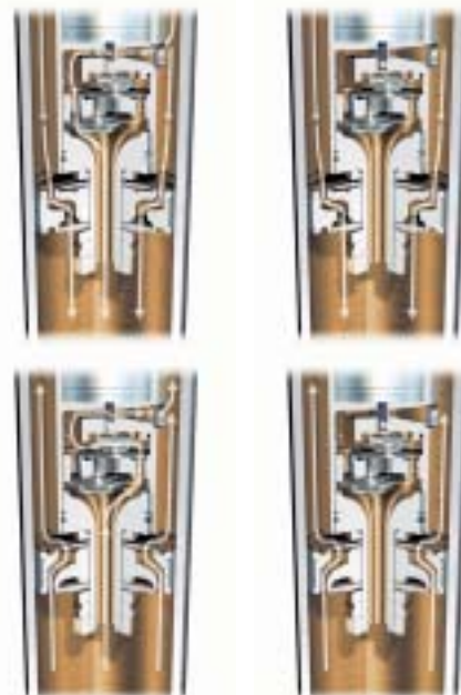
The PASM adaptive damper system is standard fitment on the Carrera S.
