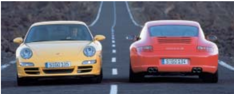
The 911 (designated 997) has reverted to a "traditional" headlight design, and the car is slightly wider at the rear than the 996. The Carrera S version (right) has quadruple tailpipes to the Carrera's two.
