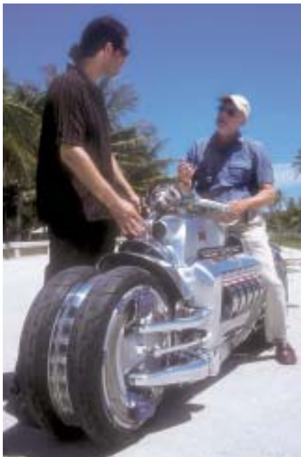
Tomahawk Product Designer, Mark Walters (left), describes the salient technology points of the four-wheel Dodge Tomahawk—an 8.3-L, 500-hp (373-kW) motorcycle—to AEI European Editor, Stuart Birch.
