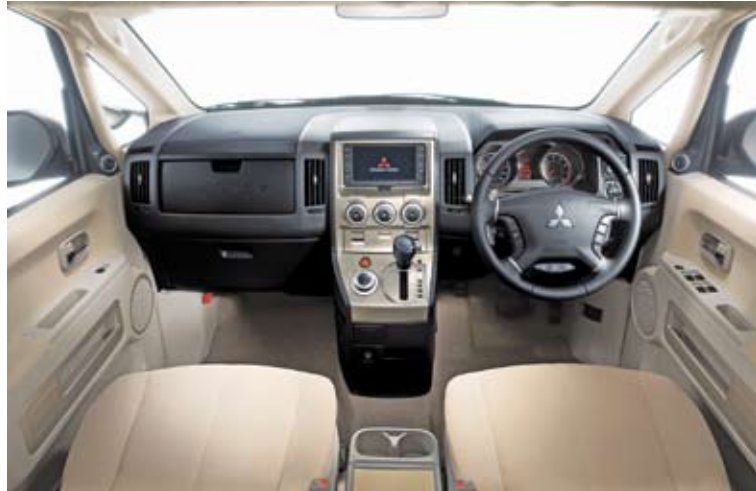
The D5 center console carries the CVT lever and AWD selector dial.
