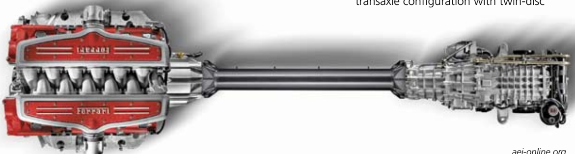
In the balance: engine and transmission layout of the new Ferrari 599.
