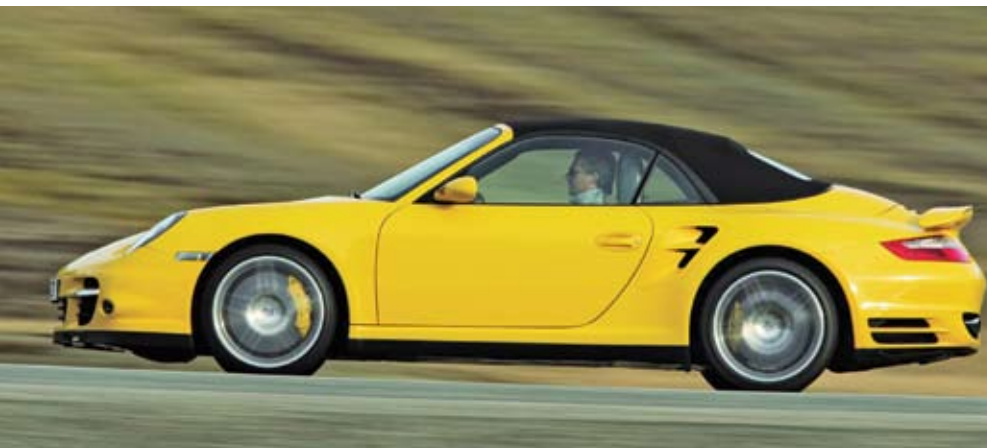
At 0.31, the Cd of the new Porsche 911 Turbo Cabriolet is identical to that of the Turbo Coupe.
