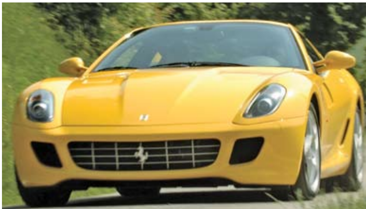
Ferrari's new 6.0-L V12 599 GTB Fiorano produces 456 kW (612 hp) and has a top speed of more than 330 km/h (205 mph).
