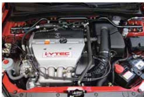
Longer duration intake valve timing and lower restriction intake and exhaust systems boost output of the RSX Type-S 2.0-L engine from 200 to 210 hp (149 to 156 kW).
