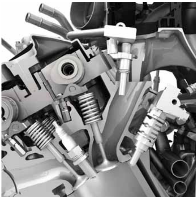
Both port and direct fuel injection are used in the IS. Shown is a cutaway of the 3.5-L V6 engine.
