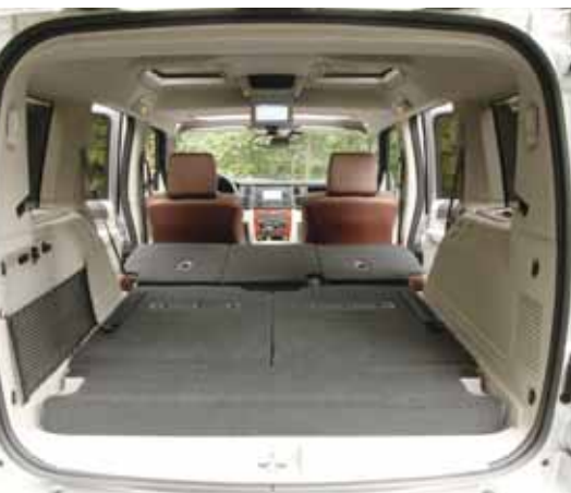
Both the second and third rows fold forward to provide a flat load floor with a cargo volume of 68.9 ft 3 (1950 L).
