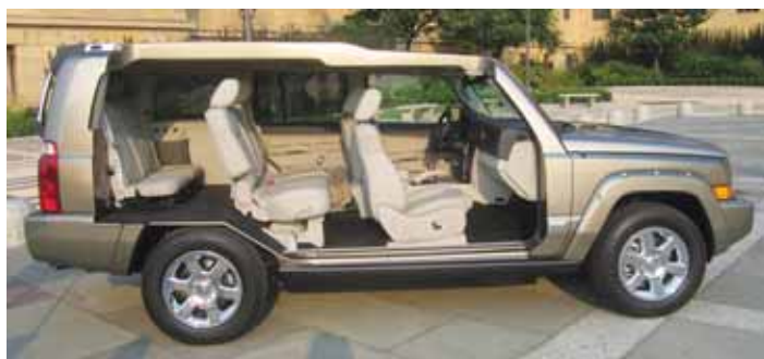
The Commander is the first Jeep to have three rows of seats. To help make room, the SUV is 2 in (51 mm) longer and nearly 4 in (102 mm) taller than the Grand Cherokee on the same 109.5-in (2781-mm) wheelbase.
