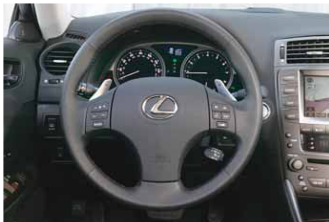
Paddle shifters on the steering column are one element of a redesigned IS cockpit.
