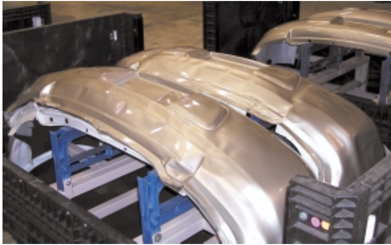
The finished fascia film, formed but flimsy, is packaged for shipping to Chrysler, where a substrate will be added.
