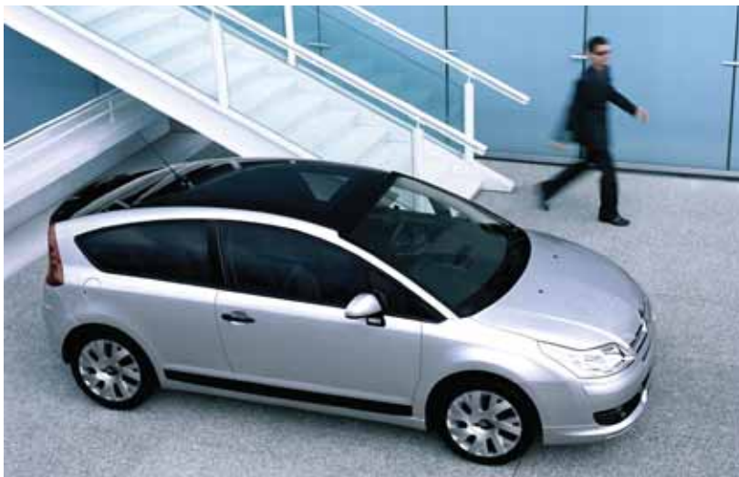
The Citroën C4, introduced at the Paris Auto Show, features a panoramic laminated glass roof with solar-absorbing nano-particles embedded in the PVB interlayer.
