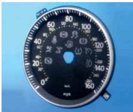
The dial ring looks like aluminum, but it is really a Bayer polycarbonate formed to look metallic.
