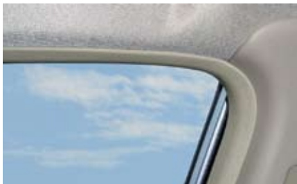
Made of NexPrene 9075A TPV from Solvay, the decorative topcoat on this door seal from Hong Yang Sealings is visible in the interior of a Mazda 323 built for the Chinese market by Haima Motor.
