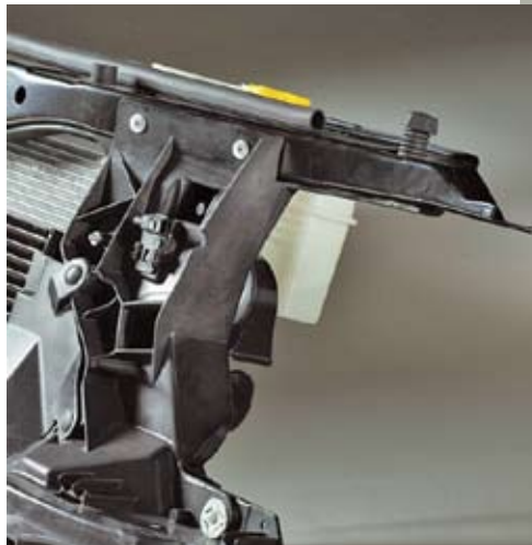
As with the 2007 Jeep Wrangler, the front-end carrier for the new Dodge Nitro (shown) uses Betamate low-energy substrate adhesive from Dow Automotive to join plastic and steel components.
