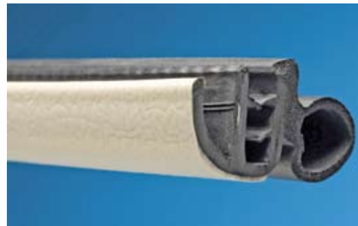
This automotive door seal features a colored topcoat of NexPrene 9075A vulcanized thermoplastic elastomer (TPV) from Solvay Engineered Polymers. The body of the seal and the foamed bulb section are co-extruded of thermoset EPDM by Hong Yang Sealings at its plant in Guiyang, China.
