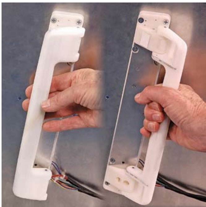
A grab handle moves into position through a combination of temperature and stiffness changes to the shape memory alloy.
