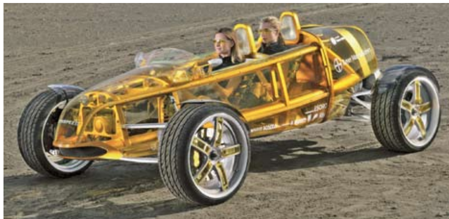
The Rinspeed eXaxis concept car features a body and floor made of Bayer MaterialScience's Makrolon polycarbonate. The two-seater has a mass of 750 kg (1650 lb).
