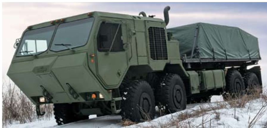
Oshkosh's third-generation Heavy Expanded Mobility Tactical Truck features a diesel-electric drive system that makes use of copper rotors for the ac induction motors.
