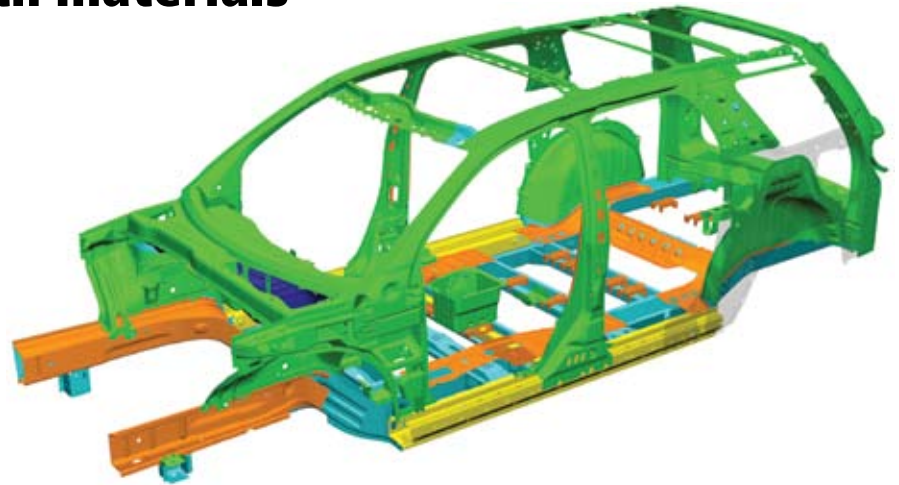
■ Ultra high-strength steel ■ Dual-phase steel ■ High-strength steel ■ Bake-hardenable steel ■ Quiet steel ■ Sheet metal
