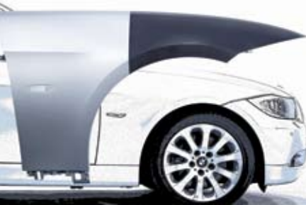
Lustran Polymers' Triax DP 3157, a mineral-reinforced, online-coatable polyamide and ABS (acrylonitrile butadiene styrene) blend, is used for the side panels of the BMW 3 Series Coupe.
