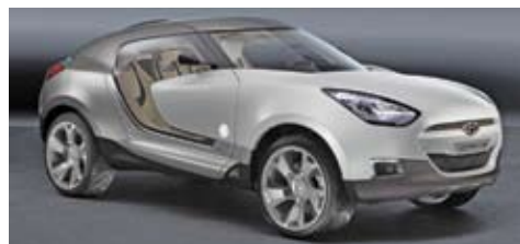
Using a thermoplastic material for a large horizontal part like the hood is one of the innovations shown in the Hyundai QarmaQ.
