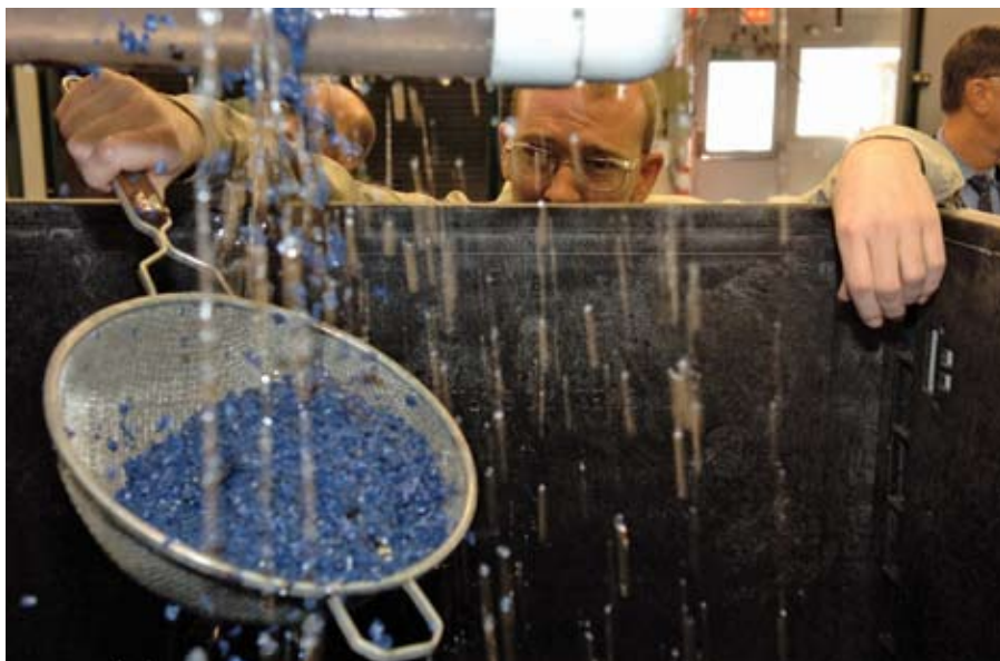
The ECO2 process is one of many USCAR VRP research initiatives under way. Here, a chemical engineer at Argonne National Laboratory sifts plastic chips ground from shredder residue, which are cleaned and sorted by froth flotation in Argonne's Pilot Plant.
