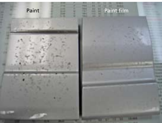
Gravelometer test samples show that paint film is more durable and chip-resistant than paint, illustrating paint film's suitability for exterior applications such as rocker panels, running boards, stone guards, fascias, bumpers, and moldings.
