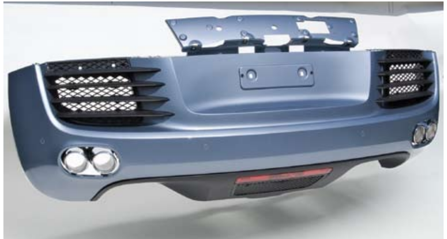
Wall thicknesses can be varied as required, those of the bumper and rear panel (the latter also produced from Bayflex 180) being between 2 and 5 mm (0.08 and 0.20 in) near the attachments.
