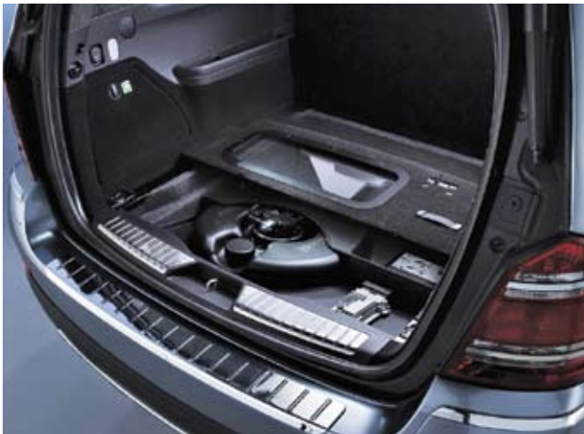
The GL320 BlueTec will package its AdBlue reservoir under the rear cargo floor, where it will carry enough fluid to last between oil-change intervals. The system consumes urea at the rate of 0.1 L per 100 km (0.1 qt per 620 mi).
