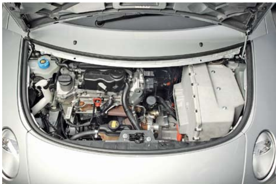
The Zytec diesel-hybrid drive was engineered to fit into the Smart ForFour engine bay.
