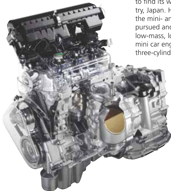
Daihatsu's 660-cm 3 inline triple is combined with a 9.4-kW electric motor and a four-speed automatic transmission in the Topaz KF.
