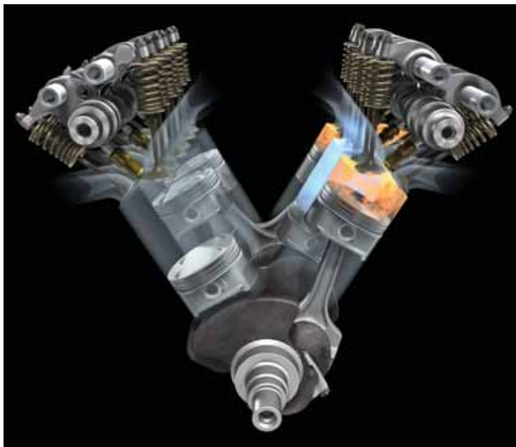
Honda's 3.0-L V6 engine features variable cylinder management and powers various car and minivan models, including the Accord Hybrid and Odyssey for North America, and the Japanese Inspire sedan and Elysion minivan.
