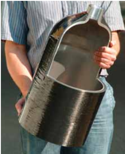
Normal operating pressure of the aluminum, carbon fiber-coated hydrogen fuel tanks of the F-Class fuel cell cars is 350 bar (5075 psi), but they have been tested at pressures exceeding 800 bar (11,600 psi).
