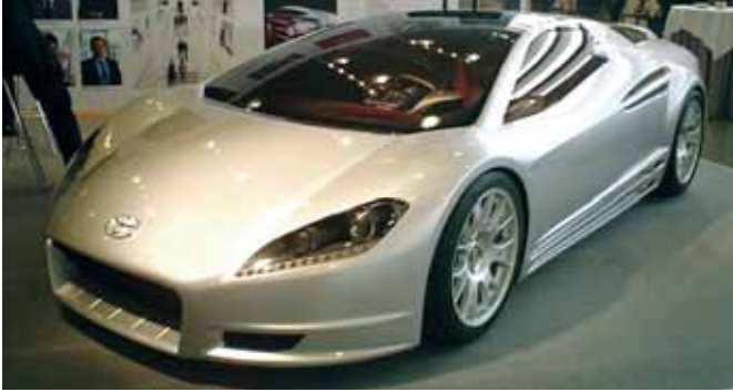
Italdesign's concept sports car uses Toyota's RX 400h-type hybrid system located behind the cockpit. An Alphard-type E-Four motor drives the front wheels.
