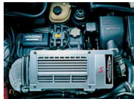
The John Cooper Works tuning kit for the Mini Cooper S increases the engine output to 154 kW (210 hp).
