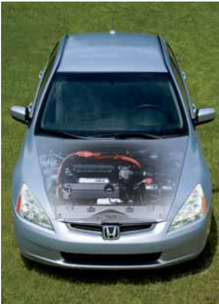
The Honda Accord powertrain combines a V6 engine with cylinder deactivation, IMA, and an electronically controlled five-speed automatic transmission.
