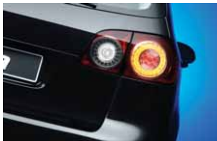
Twenty LEDs in the outer lamp rings glow yellow for the direction indicator.
