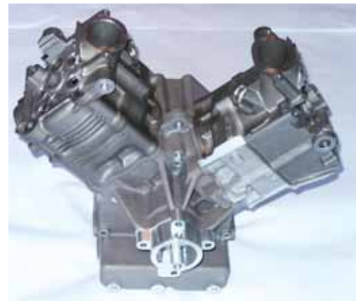
The Bruntel concept engine replaces connecting rods with planetary motion discs.
