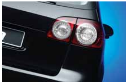
New LED technology on the VW Golf Plus does not require colored lenses.
