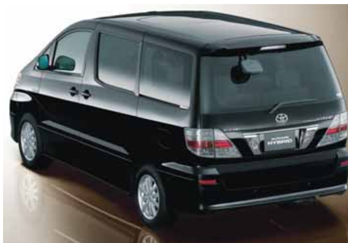
Toyota's Alphard large minivan series includes a sophisticated THS hybrid employing CVT and electric rear-wheel drive. An inline four-cylinder engine and THS-C motor/CVT drives the front wheels. A nickel metal hydride battery pack is located under the floor, and the "E-Four" motor drives the rear wheels when needed.
