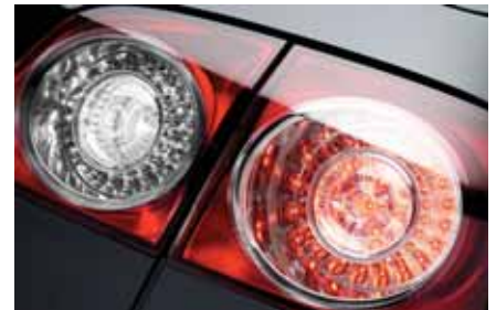
All 36 LEDs glow red for the taillight. The 16 LEDs on the inner ring light with greater intensity when the brakes are applied.
