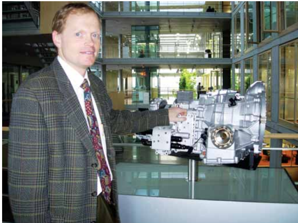
Getrag's Stephan Rinderknecht stands next to the company's DCT 477, a seven-speed dual-clutch transmission.
