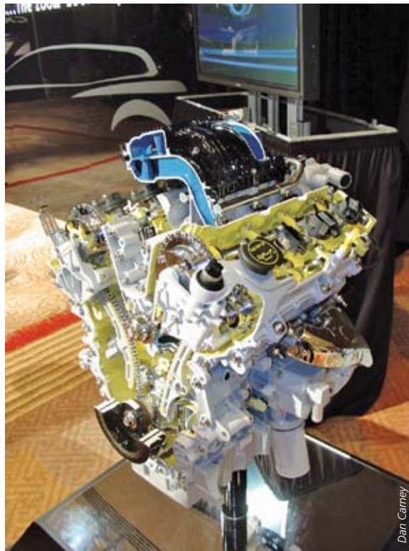
The Mazda CX-9's unique intake tract is the source of the engine's different NVH characteristics in comparison to Ford's version of the engine, according to CX-9 Product Development Engineer Stan Hortinela.
