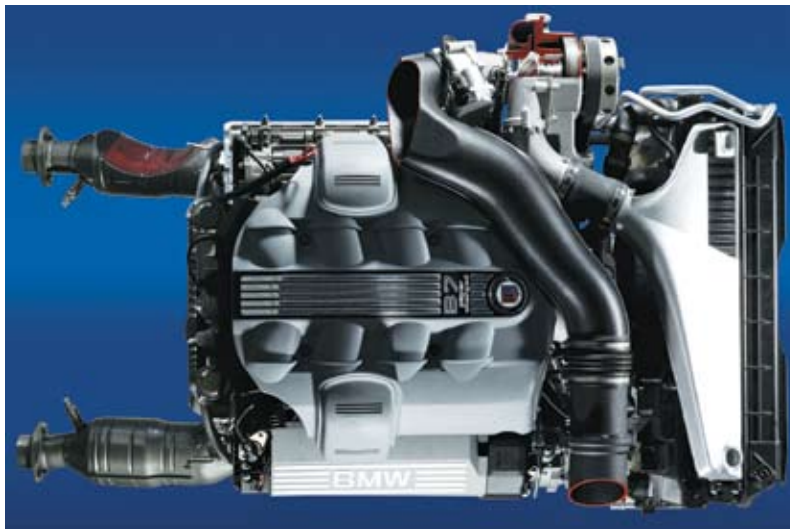
Alpina's radial supercharger, which is belt-driven through a centrifugal clutch for gradual engagement, also features a 15:1 fixed-ratio planetary gearset.
