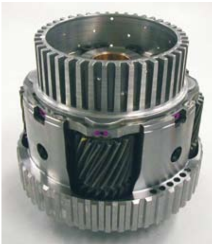
Lexus reduced the mass of the clutch hub 50% in its 8-speed automatic transmission by making it from aluminum.
