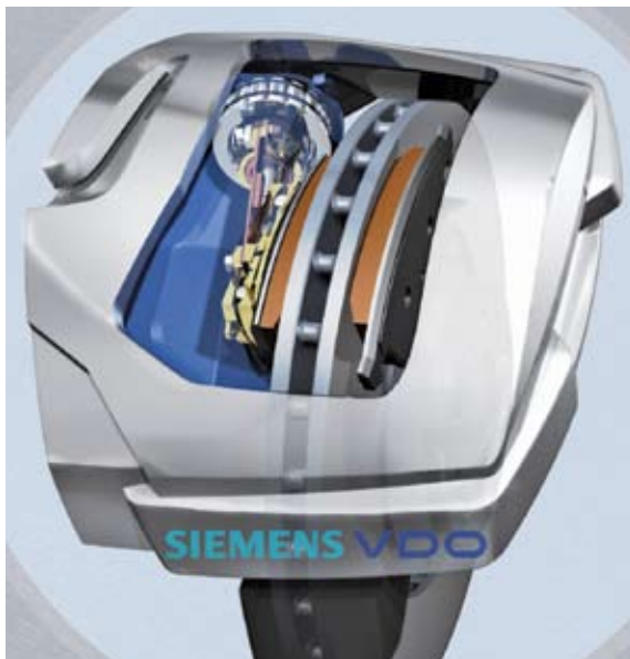
The EWB's braking mechanism takes advantage of the wedge principle's self-energizing effect.
