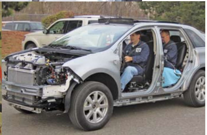
The Ford team created a working series hybrid fuel-cell demonstrator in just 100 days.
