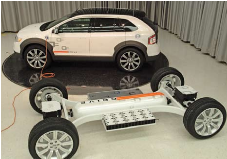
The HySeries Edge design included a central hydrogen cylinder with the fuel cell and battery pack on either side. Future HySeries powertrain architectures should allow more design freedom.
