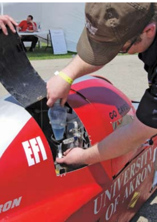
Chuck Ruggeri with the University of Akron team adjusts the 250-mL (8.5-oz) fuel bottle. All teams are required to use ISO-octane.
