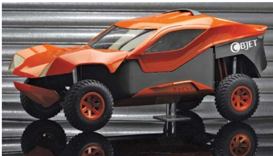
A scale model (shown) was produced for Germany's DaCar, an automotive company, via an Objet Eden 3-D machine. Once printed, the vehicle was painted to specifications.
