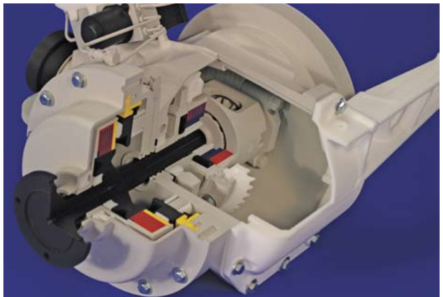
This clutch assembly, produced on a fused-deposition modeling machine from Stratasys, enabled an automotive supplier to identify and fix problems during concept design.
