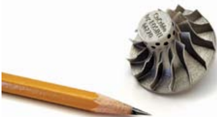
This sample geometry, based on a turbocharger-type application, demonstrates the capability of DMLS. The tiny, scaled-down part from Morris Technologies is made of cobalt chromium.
