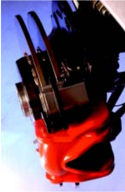
Twin floating discs are a key feature of the ADS from Delphi.
