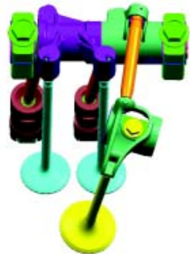
A short, nearly horizontal pushrod (orange) links the intermediate rocker arm located on the conventional rocker shaft to the stud-mounted rocker that opens the exhaust valve. A forked rocker arm operates both intake valves.
