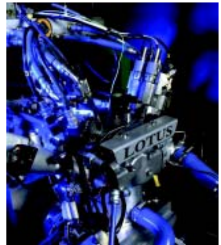
The fully variable AVT technology has a control system that achieves optimum efficiency across the entire load and speed range of the engine.
