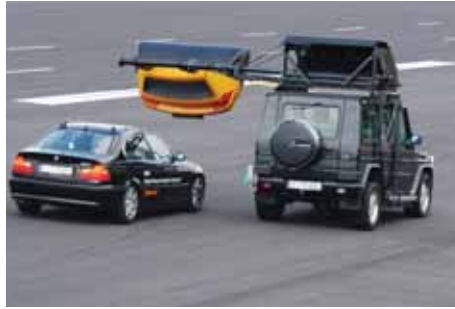
When a driver exceeds braking limits, the "leading car" flips up and out of the way in Continental's in-line driving maneuver demo.
