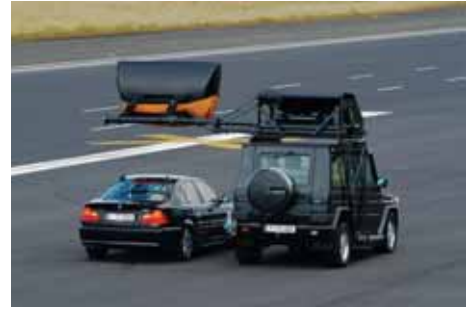
When a driver exceeds braking limits, the "leading car" flips up and out of the way in Continental's in-line driving maneuver demo.
