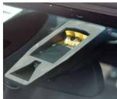
Continental's closing-velocity sensor uses pulsed laser light for short-range obstacle detection. The image on right shows the sensor attached to a windshield behind the rearview mirror.
