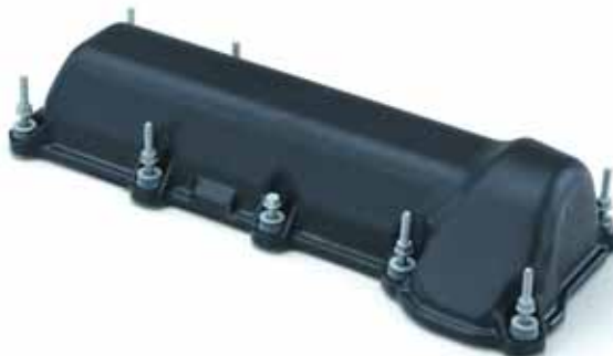
Dana's cylinder-head-cover module for the Chrysler Group's high-volume 3.7-L V6 engine has a mass savings of 4 lb (1.8 kg) per engine compared with the previously fitted steel system. It is made from a hybrid thermoset material Premix TMC (thick molding compound).
