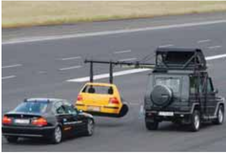
When a driver exceeds braking limits, the "leading car" flips up and out of the way in Continental's in-line driving maneuver demo.
