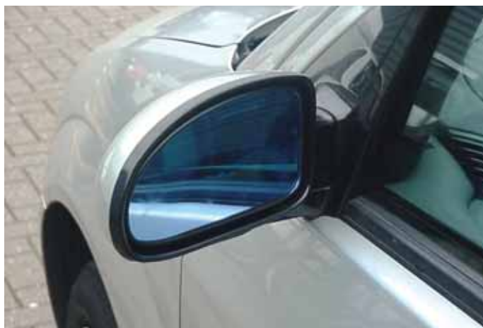
VTEC Technologies has developed a mirror reflective surface made from plastic material that is lower mass and more robust than glass.
