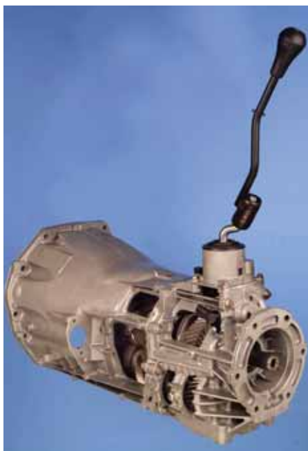
The 2005 Jeep Liberty and Wrangler get a version of the six-speed NSG 370 manual transmission first seen in the Chrysler Crossfire.
