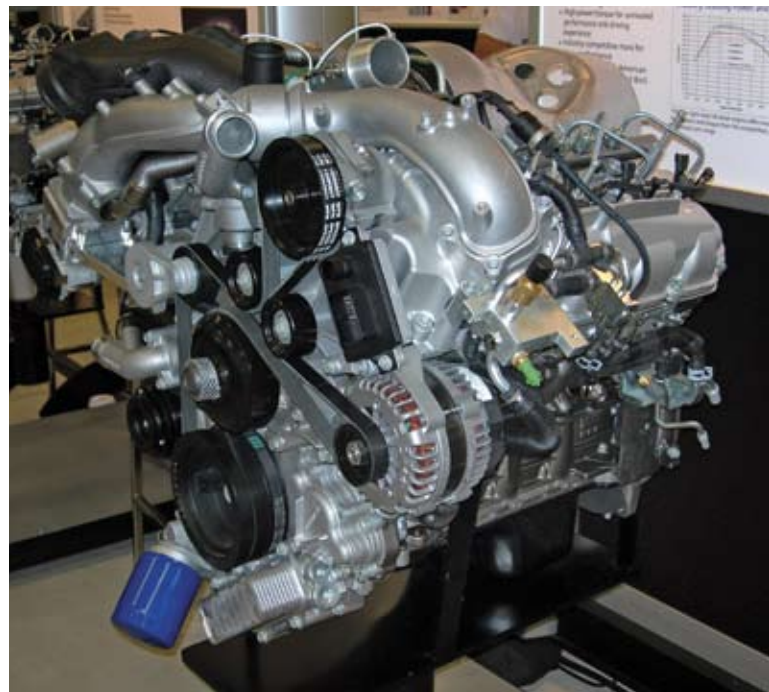
Cast-aluminum intake plumbing on the current prototype engine may be superseded by reinforced plastic before the program reaches production. The ultra-compact diesel V8 has its turbocharger hidden between the cylinder banks.
