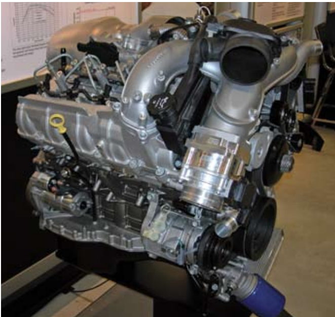
Right side of the new V8 shows lack of exhaust manifold. Intake route is straight into the top of the intake cam boxes.
