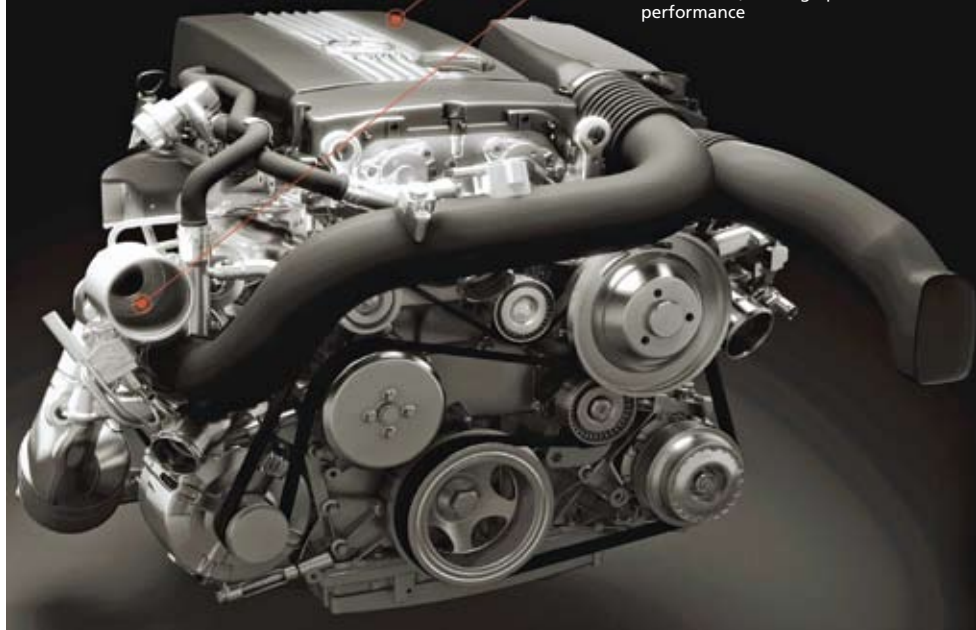
Emerging from the R&D shadows: Mercedes-Benz's DiesOtto engine melds diesel and gasoline technologies.
