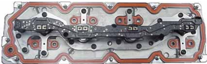
The lifter oil manifold assembly (LOMA) directs pressurized engine oil to the DRFs to deactivate and activate cylinders 1,7,6, and 4 as required by the engine controller.
