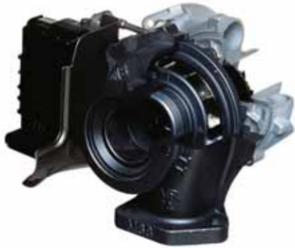
Garrett VNT (variable nozzle turbine) turbochargers, such as the third-generation version that Honeywell is supplying for the BMW 120d, adjust the gas throat section at the inlet of the turbine wheel to optimize turbine power with the required flow velocity.
