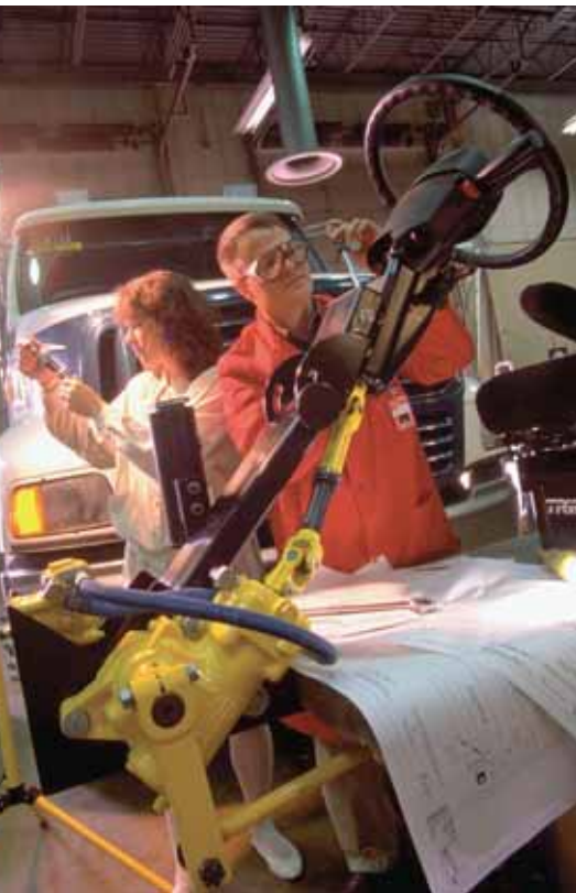
Technicians adjust a new EPHS pump for commercial vehicles. TRW claims the compact pump is the only one of its kind that prevents leakage in high-temperature applications. (Images courtesy of TRW Automotive.)
