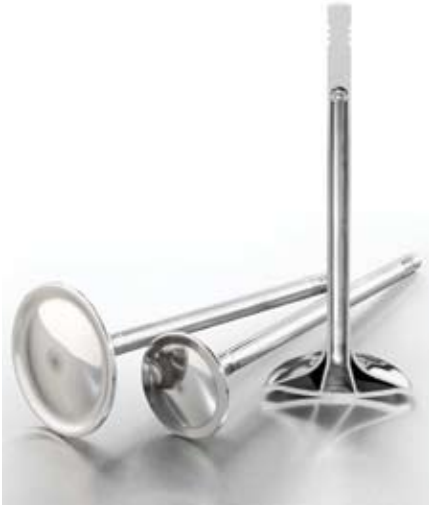
The new lightweight valves with internal sodium cooling have an extended operating range that is 50 to 100°C (90 to 180°F) greater than that of conventional valves.
