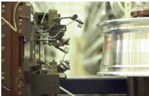
Wheel uniformity testing, done at GM's Milford Proving Ground within the Tire and Wheel Center, will not be affected by an upcoming consolidation of powertrain-related testing. But several other testing sites in southeast Michigan eventually will move into a central location in Pontiac, MI.
