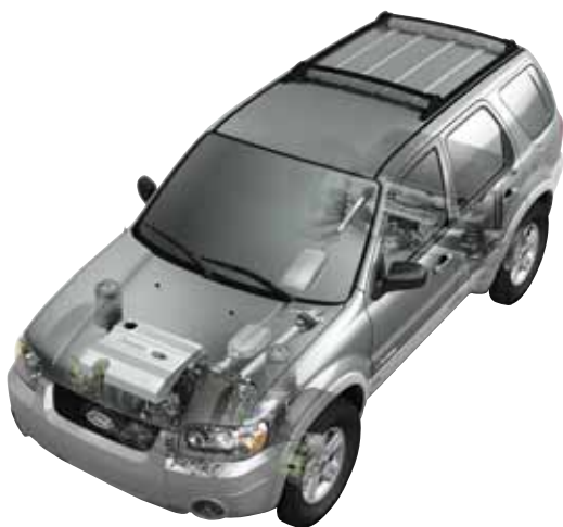
The Ford Escape Hybrid uses a Continental Teves EHB system.
