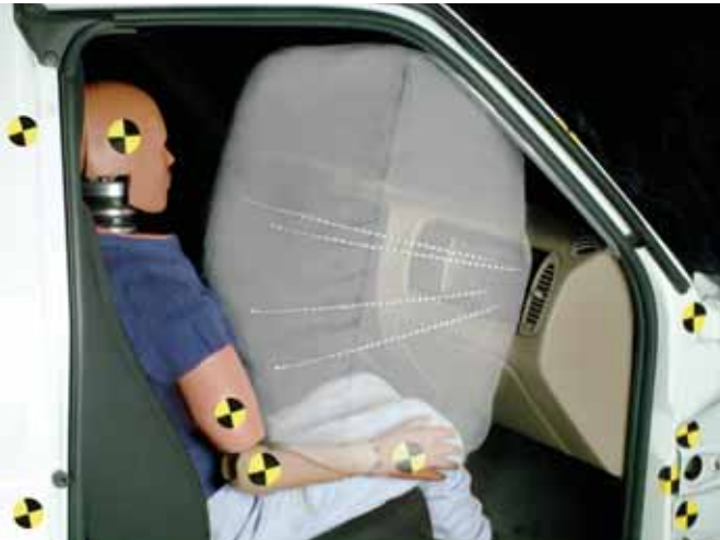
TickerTape Airbag components can be configured into a package that conforms to current production modules, consolidating the electronic circuitry, airbag cushion, and hardware components.
