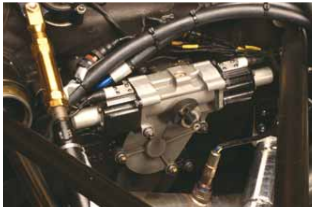
Zytek's electrically assisted Gearshift System can make four downshifts in less than one second.
