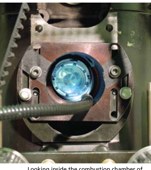
Looking inside the combustion chamber of the optical engine via a 45° mirror, which is housed inside an extended piston. The bluish light corresponds to combustion luminosity.
