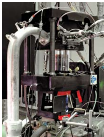
A full view of a single-cylinder diesel optical research engine within the IFP engine lab.
