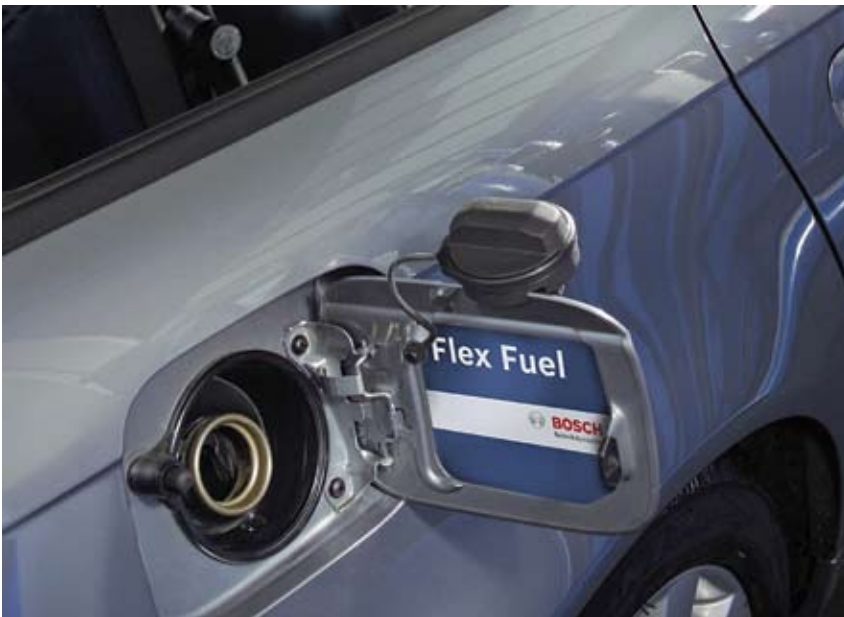
By using a flex-fuel management system from Bosch, an engine can run on gasoline, ethanol, or any mixture of those two fuels.
