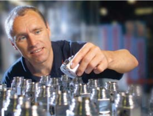
A Bosch plant in Nuremberg, Germany, manufactures many products, including single-cylinder high-pressure pumps for second-generation direct injection systems. The stainless steel pump is suitable for all grades of fuel, including ethanol.
