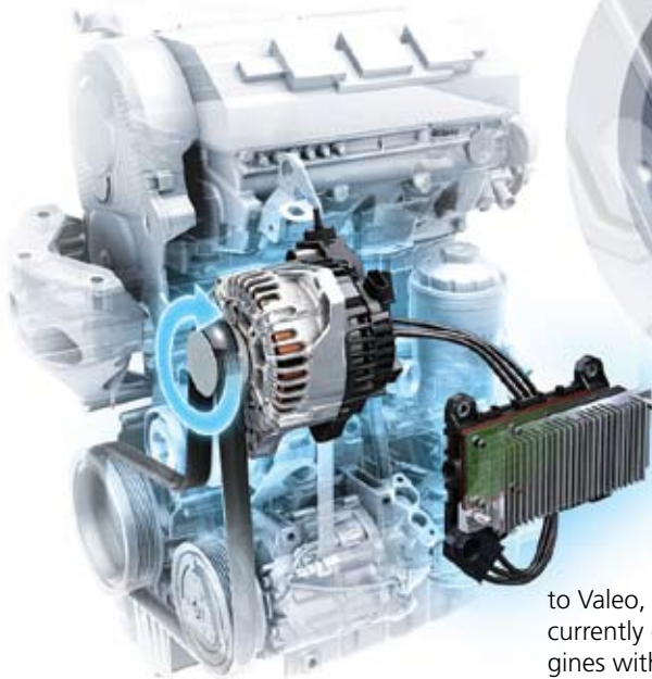
Valeo says that its StARS starter/alternator stop/start system can start diesel engines with displacements as large as 2.0 L and gasoline engines with displacements over 3.0 L.
