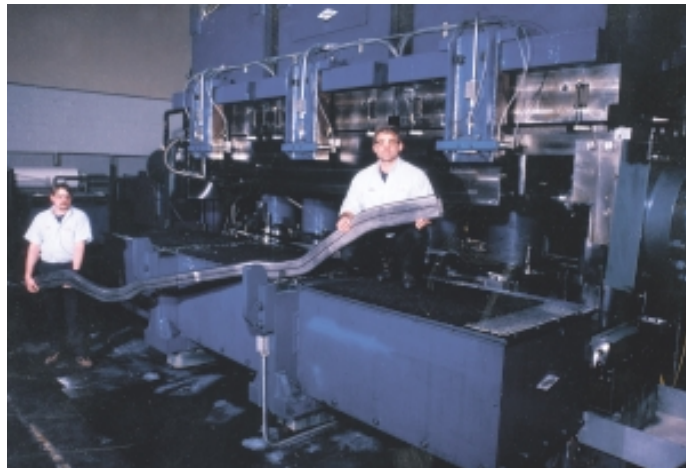
Dana's RoboClamp exerts twice the pressure of a typical hydroform press.
