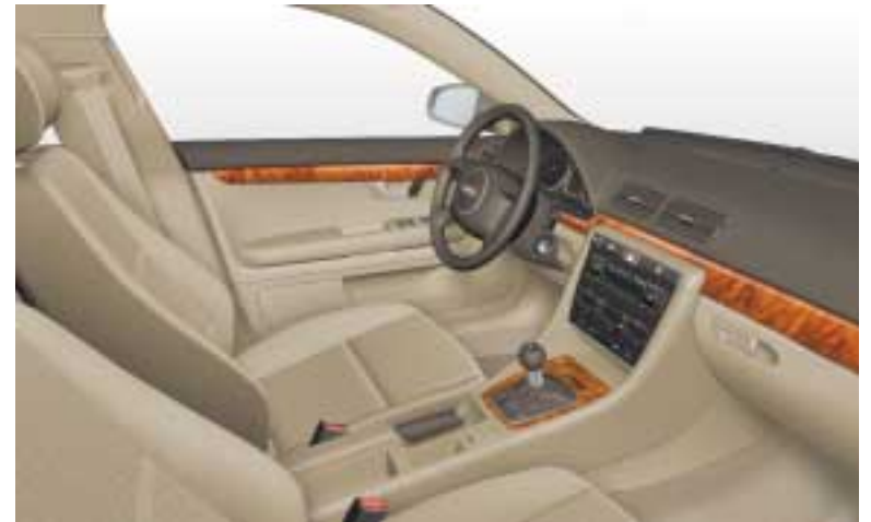
Diffuse lighting simulation is being used by Audi to enable early lighting studies to be performed in the absence of a physical mockup.
