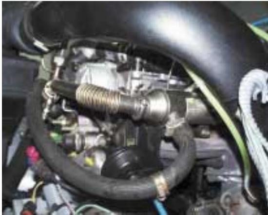
Tests have proved that an EGR cooler installed on an engine can reduce HC and CO emissions.
