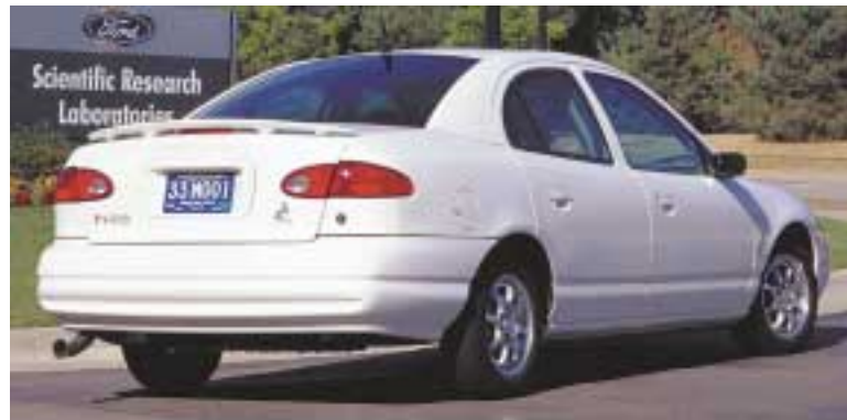
Ford's aluminum-intensive P2000 is powered by a hydrogen-fueled internal-combustion engine.
