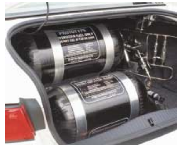
Ford's aluminum-intensive P2000 is powered by a hydrogen-fueled internal-combustion engine.
