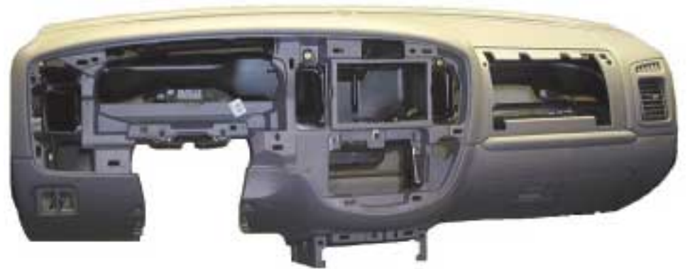
The Mazda Tribute instrument panel is constructed using Visteon's laminate injection-molding process.
