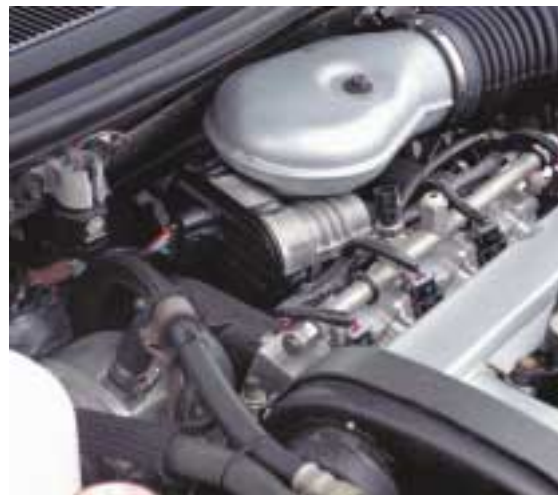
Ford's aluminum-intensive P2000 is powered by a hydrogen-fueled internal-combustion engine.
