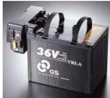
The main components of the Toyota Mild Hybrid System (shown on Japanese market Crown sedan) are a motor/generator, inverter, and 36-V lead-acid battery.
