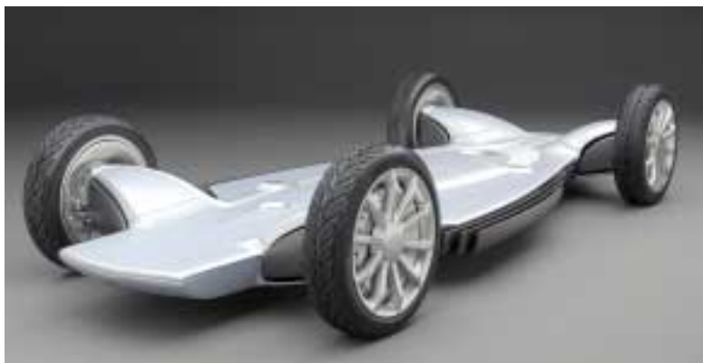
The AUTonomy's control and propulsion systems are contained within a 150 mm (6 in) thick "skateboard" chassis on which any number of vehicle bodies can be mounted.
