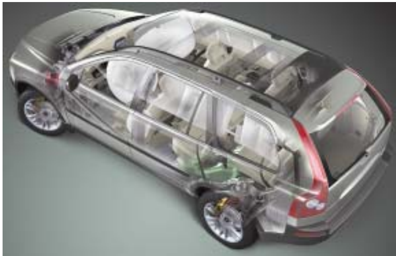
Two XC90 interior safety innovations supplied by Autoliv are seatbelts fitted with pretensioners and load limiters for every occupant as well as an inflatable curtain airbag that protects all three rows of passengers.
