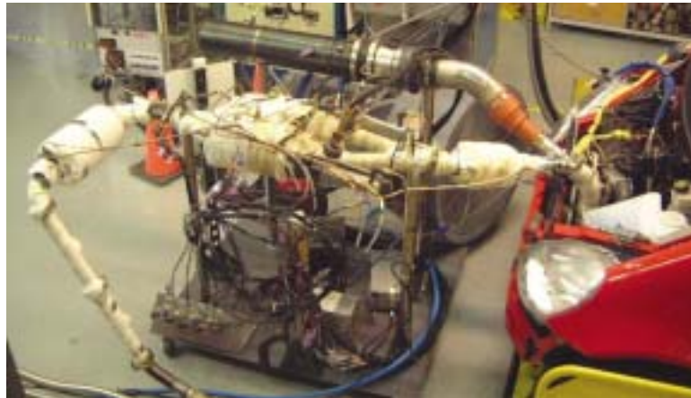
According to researchers from Cummins, Argonne National Laboratory (ANL), and the Department of Energy, one way to reduce the fuel penalty associated with NOx adsorber regeneration is to reduce O 2 flow during regeneration, accomplished via a full bypass system.
